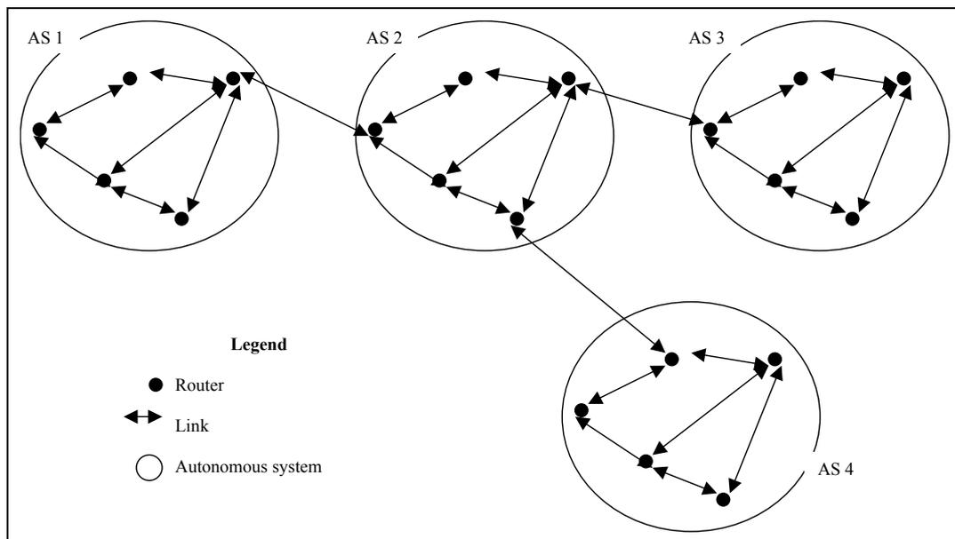
**Figure 1: Interconnection graph on router level**
